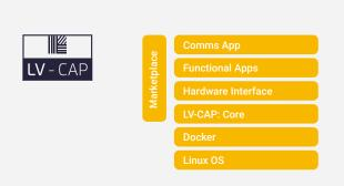
LV-CAP™ is a software platform, similar to Google's Android or Apple's iOS, but for electricity distribution substations. The platform comes with the VisNet\* Hub and is capable of hosting Applications (or 'Apps').
